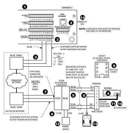
**Figure 5.** RS-232 Interface Connections (CM6700)
